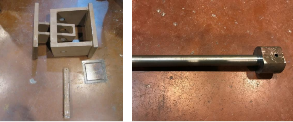
Figure 3-14: Tensile test specimen 13: (a) removed pin and (b) pin processing.
