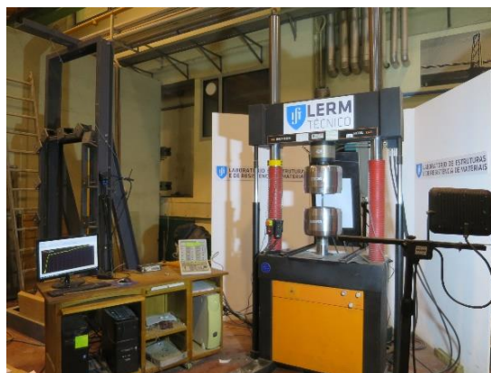
Figure 3-11: Tensile test setup at LERM.
